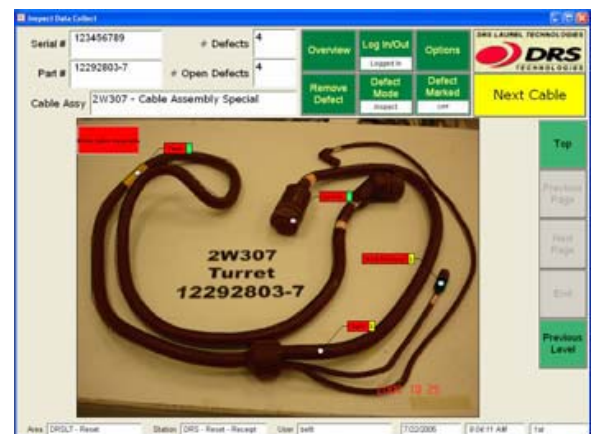
Red flags indicate repair locations
