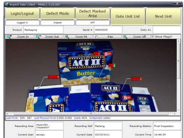
Pinpointing defects with Data Collect
