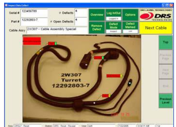
Red flags indicate repair locations
